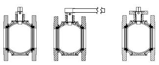
BROEN Ballomax® short ball valves without handles, with handles and with ISO-flange acc. to EN ISO 5211.
