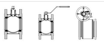
BROEN Ballomax® short ball valves without handle, with handles and with ISO-flange acc. to EN ISO 5211.
